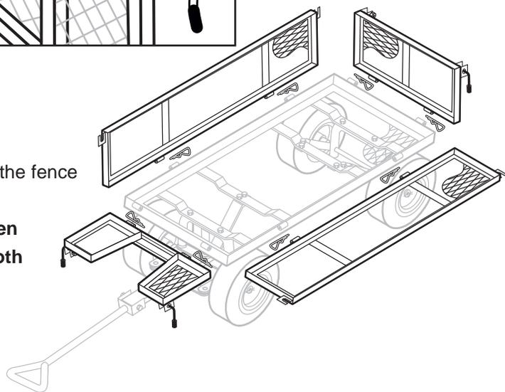
**STEP 8** Attach the pull handle to the front axle support using the 8x60mm pull handle bolt, 8mm lock nut and 8mm washer.
