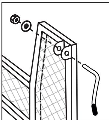
**STEP 6** Attach the lock handles onto the front and back panels using (4) 8mm lock nuts and (4) 8mm washers. **NOTE: Do not fully tighten the lock nuts. These are to be adjusted after finishing the panel assembly.**
