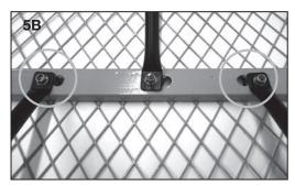
C. Next secure the rear axle assembly to the bed using M8x20 carriage bolts (2), M8 washers (2) and M8 lock nuts (2). Tighten bolts securely.
