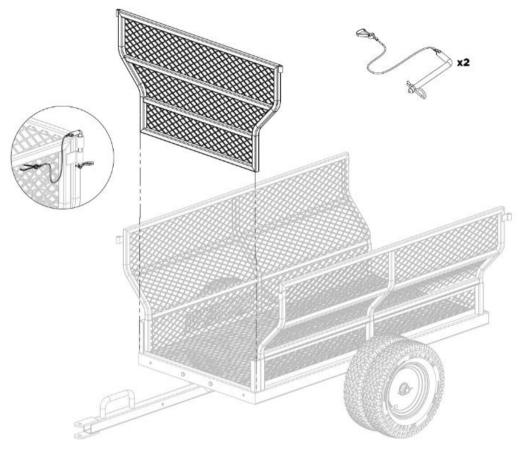
**Step 7**Attach the rear panel (1) to the trailer. Secure using tethered pins.
