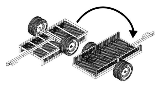
**Step 5**Attach the side panels (2) to the trailer.
