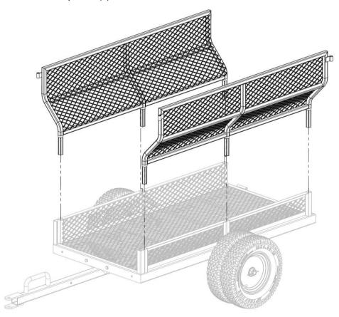
**Step 6**Attach the front panel (1) to the trailer. Secure using tethered pins.
