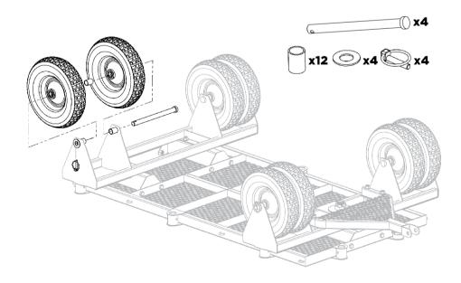
Tighten all nuts and bolts securely then flip the wagon onto the tires. Team lift is recommended.
