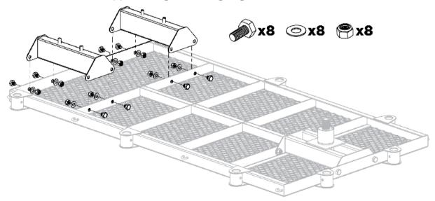
Attach the rear axle to the rear axle mounts. Finger-tighten nuts.
