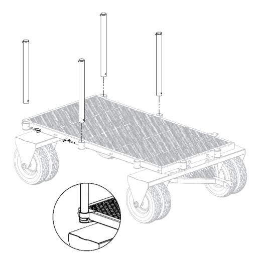
Attach the front posts (2) and the front panel (1) to the wagon. Secure using the locking pins.
