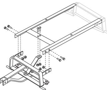
**STEP 2** The Front Axle Support is mostly pre-assembled at the factory. Please make sure all bolts and nuts assembled at the factory are tight.
