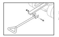
STEP 4 Attach the Pull Handle to the Front Axle Support using the 8 x 60mm Pull Handle bolt, 8mm washer and lock nut.
