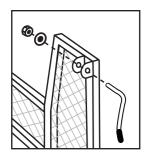
**STEP 5** Attach the Lock Handles onto the Front and Back Panels using 8mm washers and lock nuts. **NOTE: Do not fully tighten the lock nuts. These are to be adjusted after finishing the panel assembly.**
