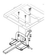
STEP 2 The front support assembly is mostly pre-assembled at the factory. Please make sure all bolts and nuts assembled at the factory are tight.
