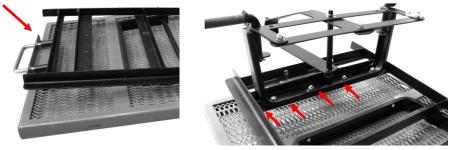
3. Attach the front struts (2) to the bed frame using M8x20 carriage bolts (2), M8 flat washers (2), and M8 lock nuts (2). Slide the M8x20 carriage bolts through the bed frame first and then through the struts.
