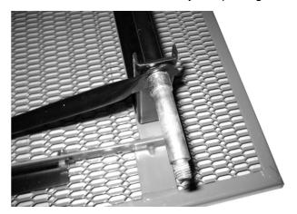
8. Place the wheels onto each axle (valve stems facing out) using the M12 flat washers (4) and M12 lock nuts (4). Tighten all nuts securely.
