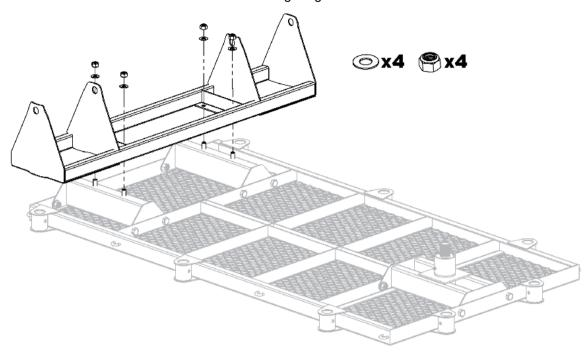
**Step 4**Attach the yoke to the front axle. Finger-tighten nuts.
